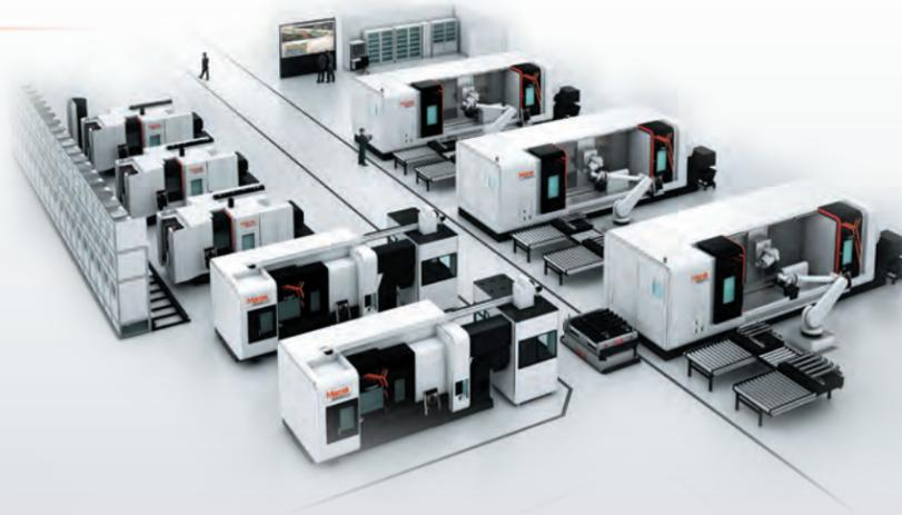
The MTConnect open communications protocol, along with process support software, monitors and harvests data from all production floor machines, cells, devices and processes. With PCs, smartphones and tablets, management and manufacturing teams access real-time data for improved production efficiency and responsiveness. Customers can achieve these same results in their shops, and Mazak not only makes it possible: It shows customers the way.
