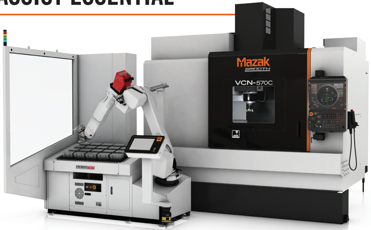
VCN-570C w/ RoboJob Mill Assist
