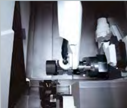
Unloading finished workpiece
